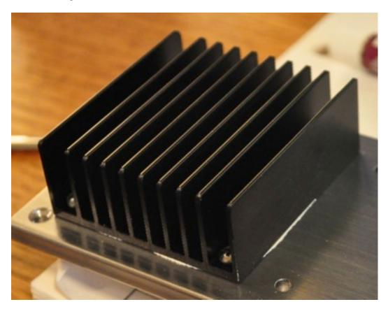
There was additional squeeze out for a day or so as the pressurized thermal grease made it's way to the edges of the heat sink. This resulted in a good thermal bond. Here is a picture of the entire "heat sink unit" all assembled showing both sides.
