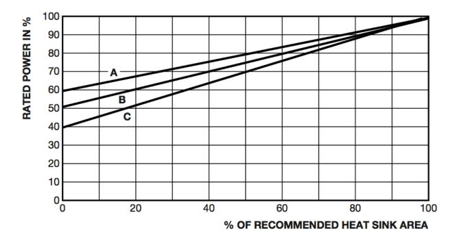
The "C" curve is the one for the TMC50 series. We can quickly see that at 6% of heat sink area the real power rating is only about 44% or  $\approx$ 22W. This is not much better than leaving the power resistor unmounted in open air. If I only used two of the four loads, I can assume 12% of the required heat sink area. However, this only is still only about 47% or  $\approx$ 23.5W.
