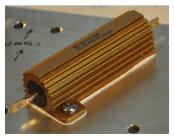
This is just about the right amount of squeeze out you want to achieve. Once the four resistors were mounted I went to work on the heat sinks. When Applying grease to these units I intentionally held back from the edges by about 1/8th of an inch. This is because I did not want an excessive amount of squeeze out to have to clean from the top. Here is how I applied the thermal grease to the heat sinks.
