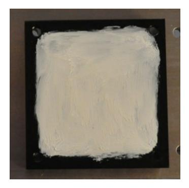
This is good for minimizing the squeeze out and still getting good coverage. When the heat sinks were mounted, the squeeze out looked like this.
