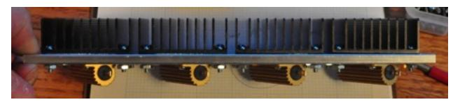
Here the heat sinks are on the top of the plate; held in place by four 6-32 screws for each. The power resistors are mounted to the underside, one under each heat sink, with 1/4'' 4-40 screws into tapped holes. This configuration assures a good short thermal path between the power resistors and the heats sinks.
