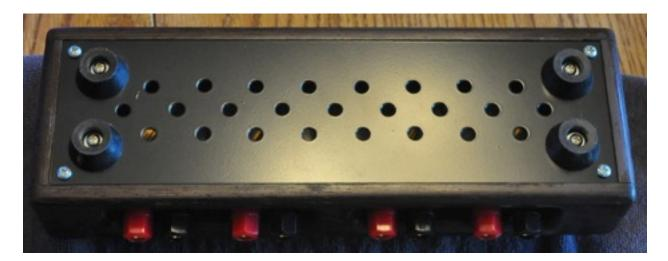
These 25 holes are the equivalent of a 1.2 square inch hole in the base plate. This should be more then sufficient to keep it from getting too hot inside the chassis.
