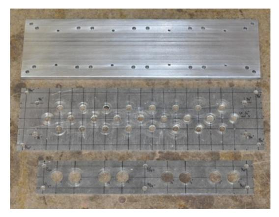
The main heat sink is sized for four VHS-95 Extruded heat sinks from V Infinity (<u>www.v-infinity.com</u>) on top and four TMC050 wire wound power resistors from Vishay (<u>www.vishay.com</u>) on the bottom. However, this was not my original configuration. Perhaps I should explain.
