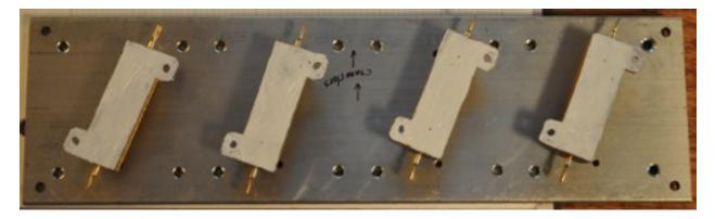
These are going to be in the case so a little squeeze out is acceptable. The object is to get just enough thermal grease on the surfaces to ensure that there are no unfilled voids between the two
